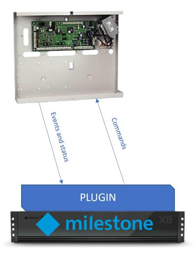
Due to this architecture configuration, the panel has to be equipped with an Ethernet module (E080) in order to communicate with the Plugin.
