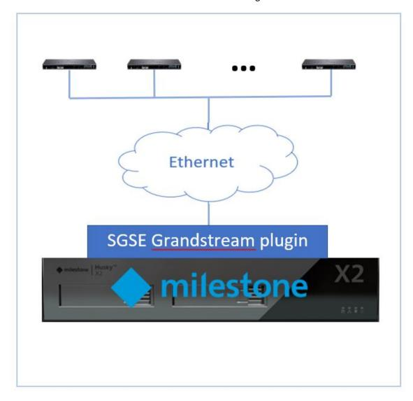
Through the Ethernet network, the plugin connects with the switchboard to automatically import the paging groups and the extensions that are configured in the IP PBX Grandstream UCM6510. The Grandstream panel must be configured so that communication between the Grandstream switchboard and the plugin is possible, and it is possible to make status requests from the different extensions. The basic configuration required to work with the plugin will be described later in this document.
